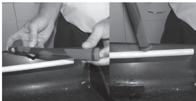
Step 8 - Align 'tick' marks on each end of grip and center line with square club face.
